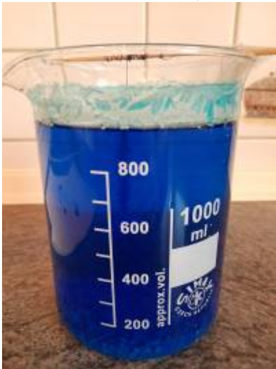
Picture 1.7: Seed crystal in solution
