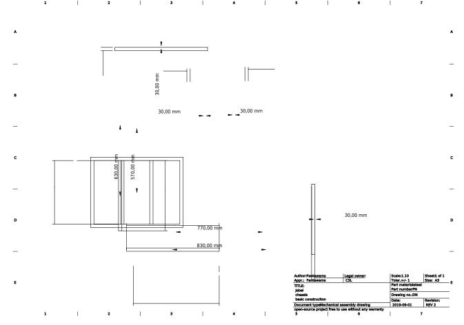
The basic construction is made out of steel with 2mm strength. We cut the 30mm pipes to the right sizes.
