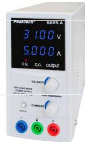
Verify that the device you want to hook up is not powered separately! The green connector is directly connected to the ground on the lab power supply's plug. Only use it for grounding if necessary, as wrong usage could flip the breaker. Do not short the connection, this could break the internal breaker of the lab power supply, and is very dangerous and might result in 3rd degree burns.
