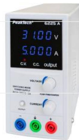
Verify that the device you want to hook up is not powered separately! The green connector is directly connected to the ground on the lab power supply's plug. Only use it for grounding if necessary, as wrong usage could flip the breaker. Do not short the connection, this could break the internal breaker of the lab power supply, and is very dangerous and might result in 3rd degree burns.
