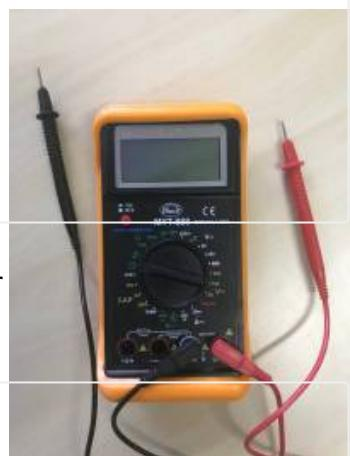
Turn on the device with the red button on the left, connect the leads to their corresponding plugs on the device. Black lead usually goes to COM.
