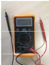
Turn on the device with the red button on the left, connect the leads to their corresponding plugs on the device. Black lead usually goes to COM.
