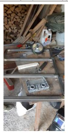
We welded a basic construction out of the steel. As we decided to use only to motors for the first version, we had to improvise a fix for the hoverboard motors. There is a height difference of 9cm between the front wheels and the hoverboard wheels. To have a aligned surface later on, we welded 3 spare pieces together.
