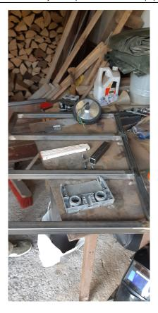
We welded a basic construction out of the steel. As we decided to use only to motors for the first version, we had to improvise a fix for the hoverboard motors. There is a height difference of 9cm between the front wheels and the hoverboard wheels. To have a aligned surface later on, we welded 3 spare pieces together.
