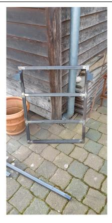
To be able to mount the front wheels and the hoverboard motors onto the chassis, we are using M8 screws. So we drill all the necessary holes into our chassis.
