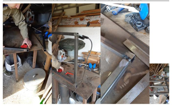
As we decided to use only 2 motors for the first version, we had to improvise a fix for the hoverboard motors. There is a height difference of 9cm between the front wheels and the hoverboard wheels. To have an aligned surface later on, we welded 3 spare pieces together to fix the hoverboard motors onto the chassis.
