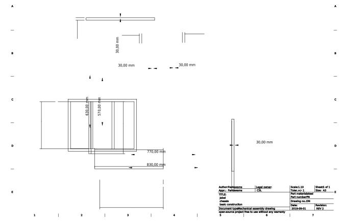
The basic construction is made out of steel with 2mm strength. We cut the 30mm pipes to the right sizes.
