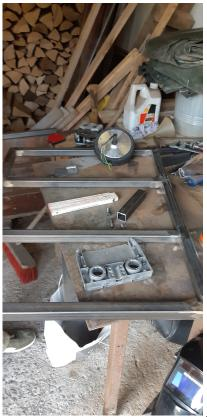
As we decided to use only 2 motors for the first version, we had to improvise a fix for the hoverboard motors. There is a height difference of 9cm between the front wheels and the hoverboard wheels. To have an aligned surface later on, we welded 3 spare pieces together to fix the hoverboard motors onto the chassis.
