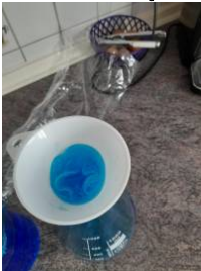
Picture 1.11: Filtering with cotton pad
