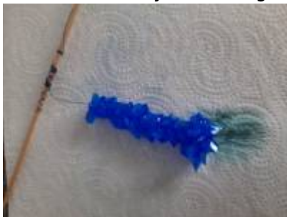
Picture 1.9: Polycrystals of Copper(II)-sulfate pentahydrate
