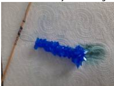
Picture 1.9: Polycrystals of Copper(II)-sulfate pentahydrate
