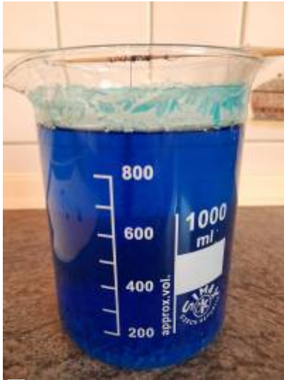
Picture 1.7: Seed crystal in solution
