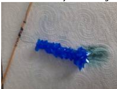
Picture 1.9: Polycrystals of Copper(II)-sulfate pentahydrate
