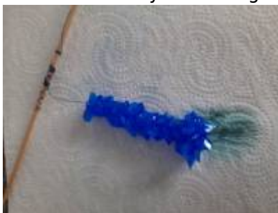
Picture 1.9: Polycrystals of Copper(II)-sulfate pentahydrate
