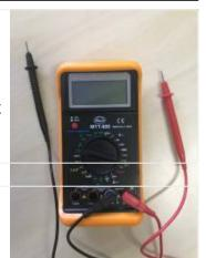
If you measure voltage or resistance, polarity can be swapped (but shouldn't for voltage). If the polarity is swapped for voltage, then the multimeter shows a negative value. Never swap polarity for measuring amperage. A diode only let's the current flow in one direction so try swapping the polarity if the diode drop is out of range.
