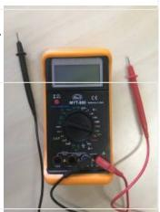
If you measure voltage or resistance, polarity can be swapped (but shouldn't for voltage). If the polarity is swapped for voltage, then the multimeter shows a negative value. Never swap polarity for measuring amperage. A diode only let's the current flow in one direction so try swapping the polarity if the diode drop is out of range.
