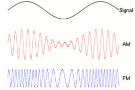
In analog frequency modulation, such as radio broadcasting, of an audio signal representing voice or music, the instantaneous frequency deviation, i.e. the difference between the frequency of the carrier and its center frequency, has a functional relation to the modulating signal amplitude.
