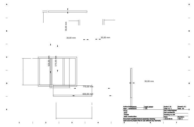
The basic construction is made out of steel with 2mm strength. We cut the 30mm pipes to the right sizes.
