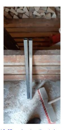
Than we welded 2x83cm pipes and 2x57cm pipes together, to have an chassis. The other 2 57cm pipes are used to have a sturdier chassis. It will be used to fix the batteries, mainboard and of course our bearing surface.
