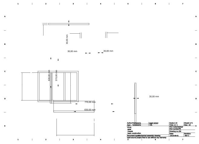
The basic construction is made out of steel with 2mm strength. We cut the 30mm pipes to the right sizes.
